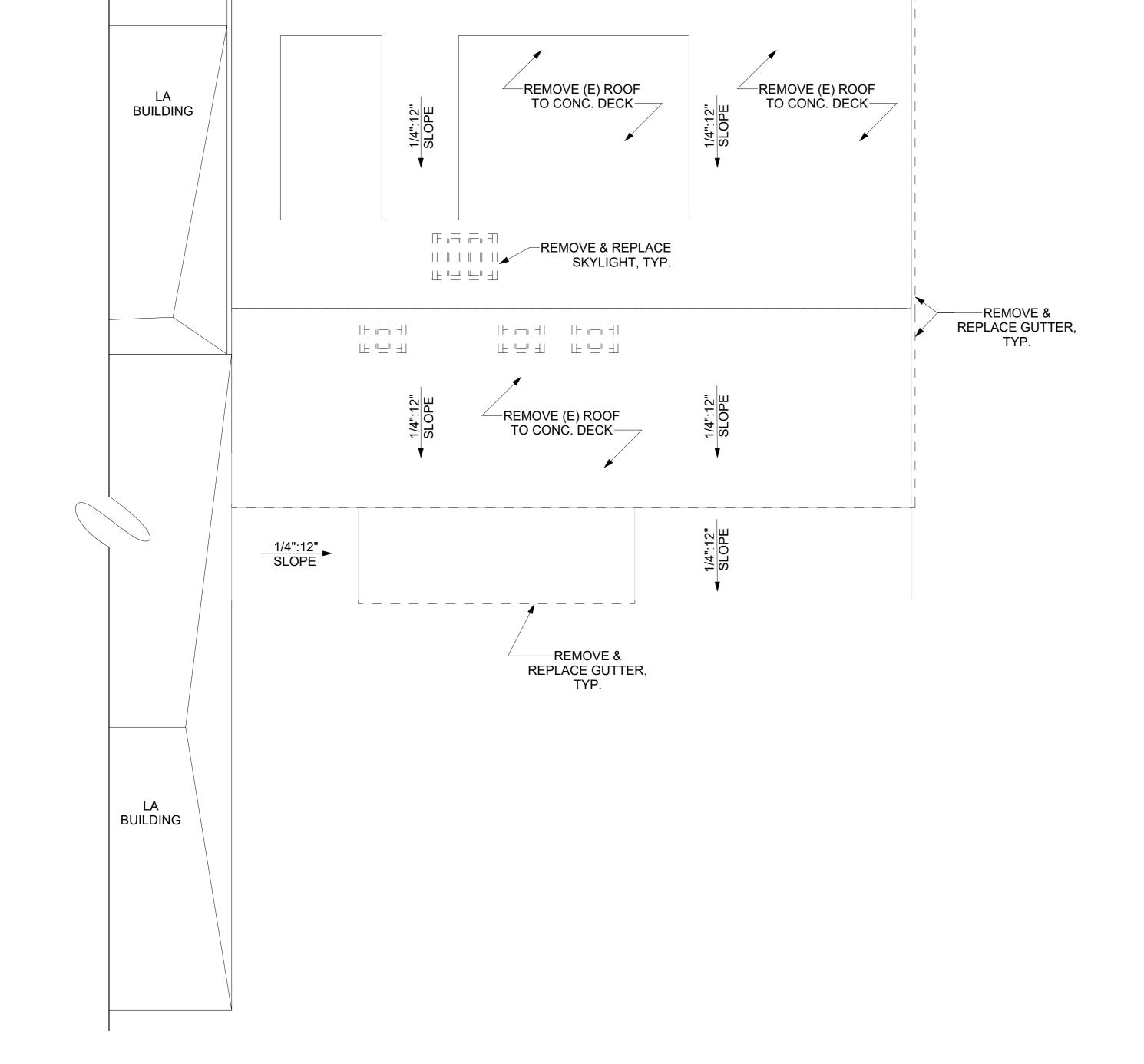
MU BUILDING - DEMOLITION ROOF PLAN
